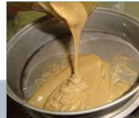
Filtration of the emulsion based on the “Eximol” emulsifier through the strainer – sediment is not present
