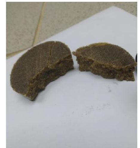
5. Physical appearance of the filtration crust of the sand, cross section
