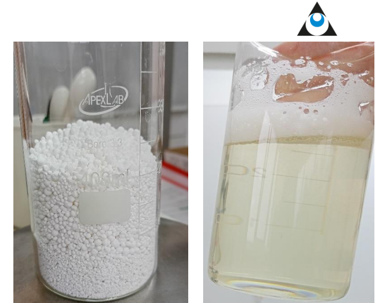
Physical appearance of “TITAN” based jamming fluid
