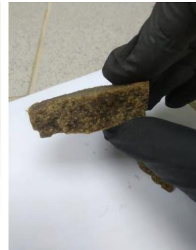
4. Physical appearance of the filtration crust of the sand, cross section
