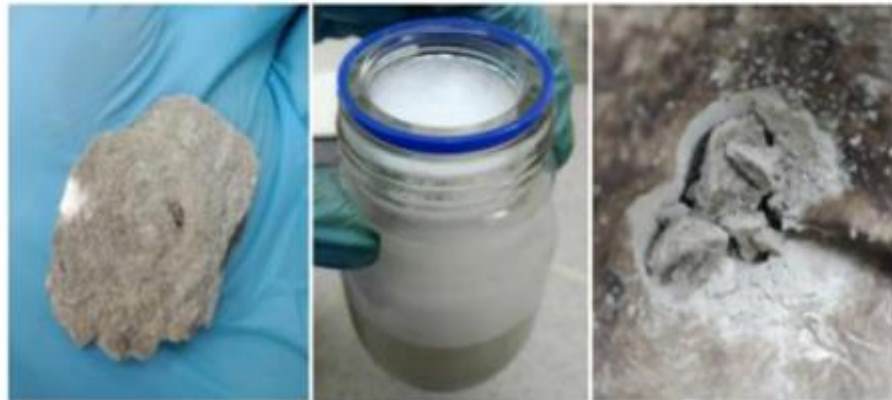
3. a) Samples of the geomaterial before dissolution in the acid composition; b) samples of the geomaterial in acid compositions “DISKOR-20”; c) samples of the geomaterial at the end of the tests
