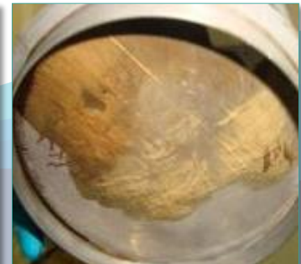
Filtration of the emulsion based on the “Eximol” emulsifier through the strainer – sediment is not present
