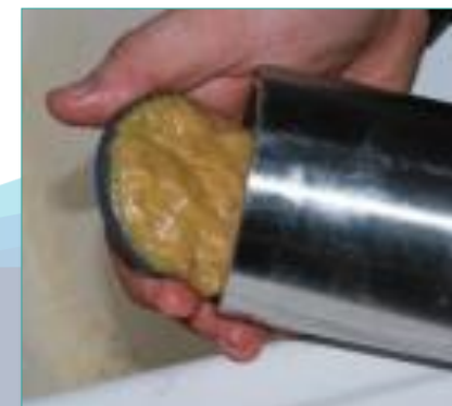
Appearance of filtration crust of the blocking composition “UNISOLT”
